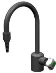
Delonized Water Gooseneck Faucet PVC faucet for distilled water. 6" rigid gooseneck. 3/8" NPT. Cat. No. 50043
